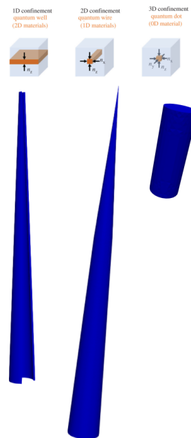
Figure 1: The three structures: the nanowire (middle), the quantum well (left) and the quantum dot (right).
